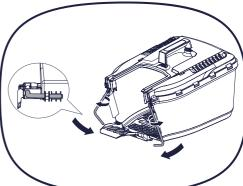
iii. Lift up the safety guard before assemble the grass bag. Hang the collection bag on the mower
